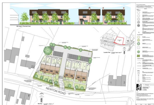
The final scheme layout showing a continuous frontage and parking to the rear
